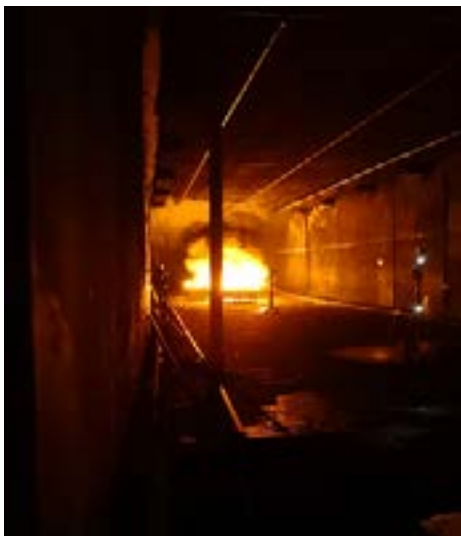
Full scale tunnel fire testing at APPLUS test center in San Pedro de Anes, Spain
