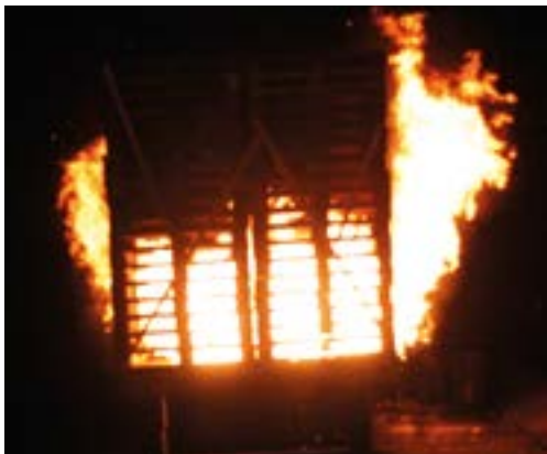
Full scale tunnel fire testing in Runehamer test tunnel, Norway
